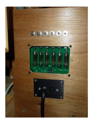
The five section switches are at the top. (Yes, I know there are six, but that is for any future change of plan). In each case the centre position, as shown, is *off*, and down is *on*; except for the left hand section 1 switch where centre is *off*, down is *on* for DCC, and up is *on* for DC. The cable at the front connects to the Powercab, and the H&M controller is wired in at the back. That is all there is to it. Oh really - so what is that green board in the middle with the tubes on it?
